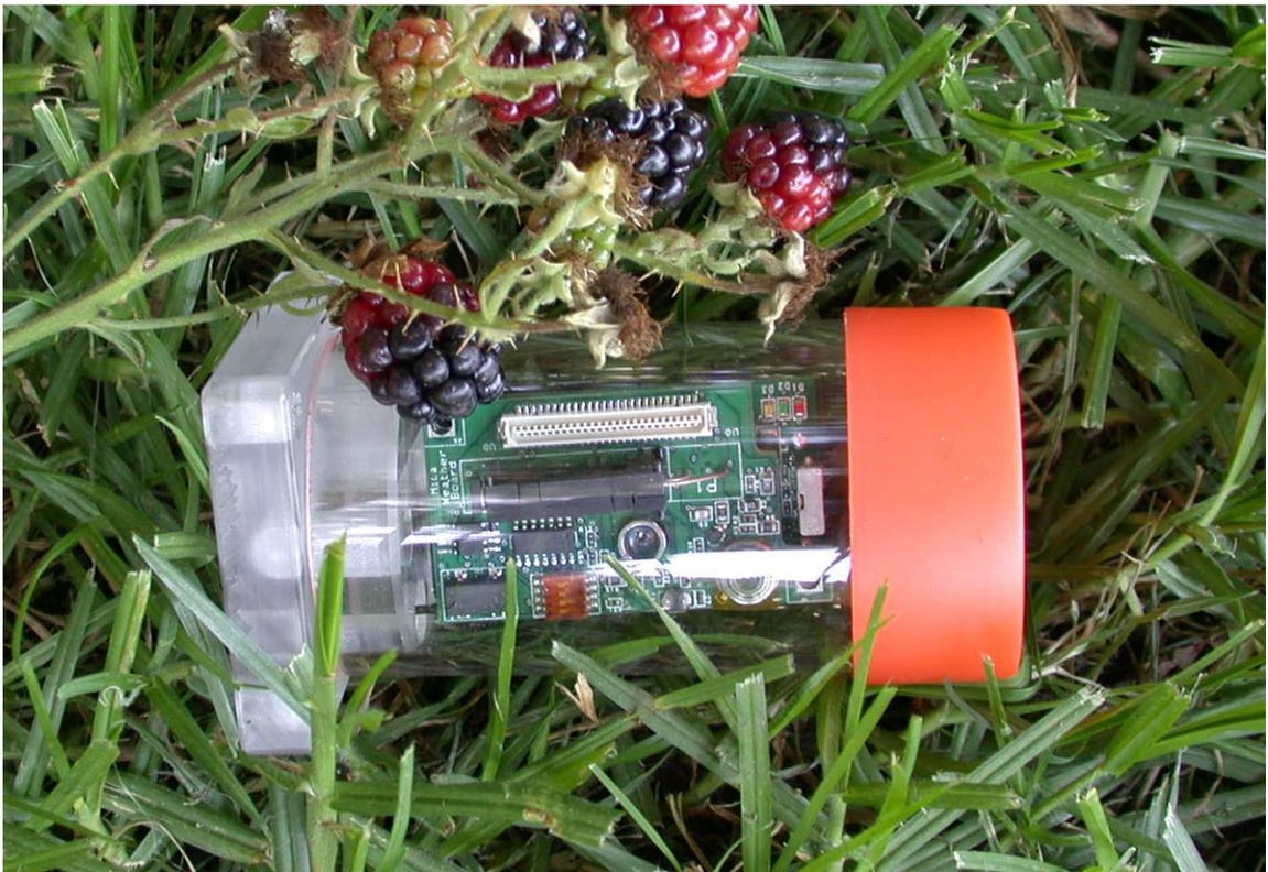
Figure 4: Acrylic enclosure used for deploying the *Mica* mote.
